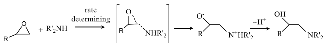
Scheme 3-3 General mechanism for epoxy-amine curing [52]
