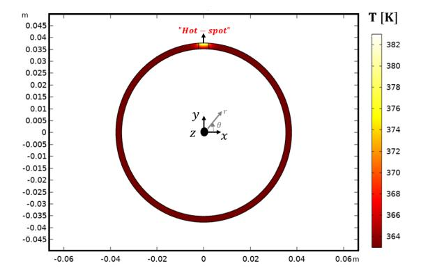
Figure 4.2: Ring surface temperature distribution
