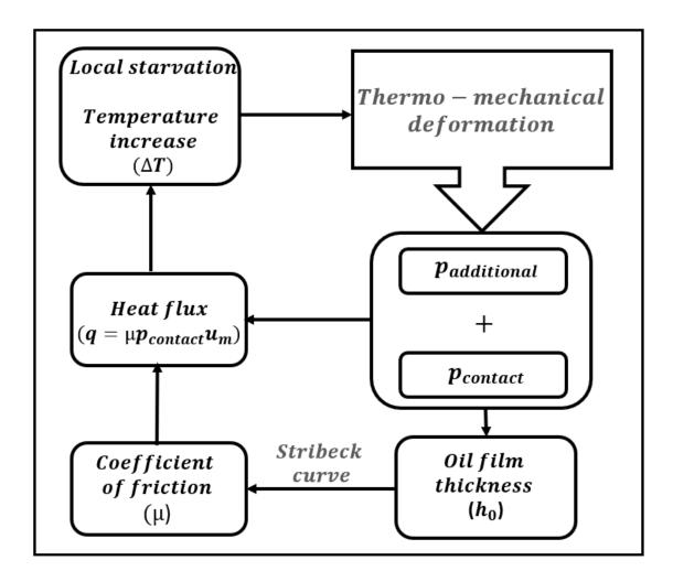
**Figure 4.1:** Algorithm of the thermo-mechanical loop
