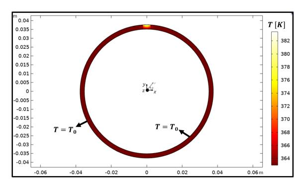
**Figure B.4:** Temperature distribution of a ring (2D model analysis)
