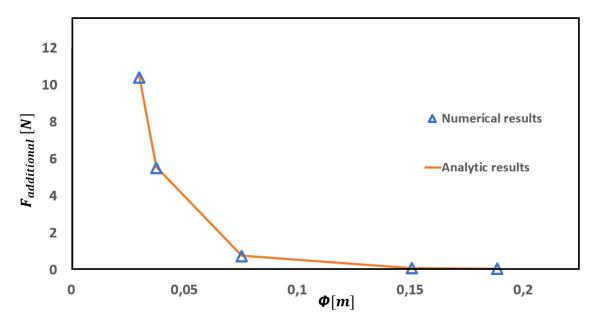
**Figure 4.4:** Numerical and analytic results of the additional load as a function of the ring diameter
