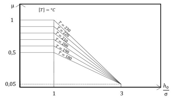
**Figure 4.6:** Stribeck curve: the coefficient of friction as a function of the temperature and the ratio of the film thickness over the surface roughness when the temperature is higher than the limit temperature
