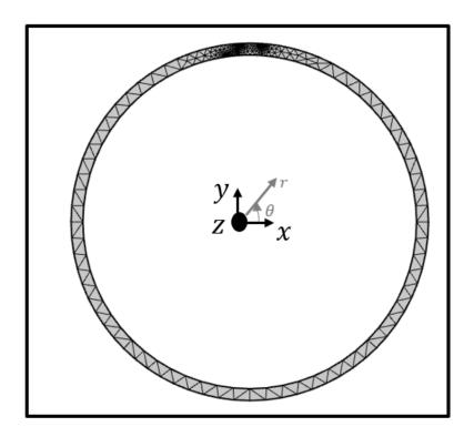
Figure B.7: Case 1: mesh grid of the ring surface
