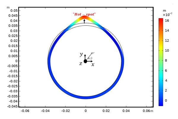
**Figure 4.3:** Ring surface deformation as a result of the surface temperature distribution shown in figure 4.2
