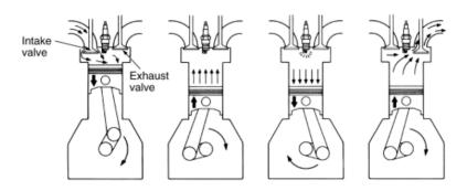
Figure 1: Four-stroke operating cycle of an ICE engine [1]
