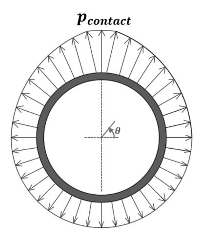
Figure 3.4: Radial pressure distribution of a piston ring
