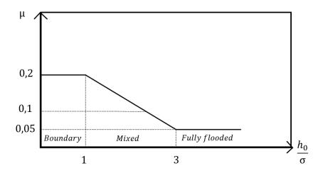
**Figure 2.13:** Stribeck curve: coefficient of friction as a function of the film thickness over the surface roughness
