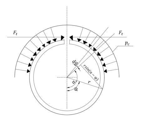
Figure D.1: Constant contact pressure distribution
