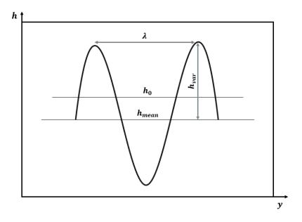
**Figure 2.8:** Oil distribution geometry
