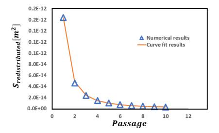
**Figure 3.17:** Numerical results and curve-fit surface redistributed as a function of the number of passages
