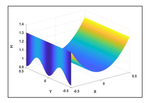
Figure 3.10: Lubricant geometry distribution before the ring passage along the liner
