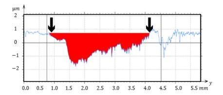
**Figure 2.3:** Wear measurement in the y-direction [7]
