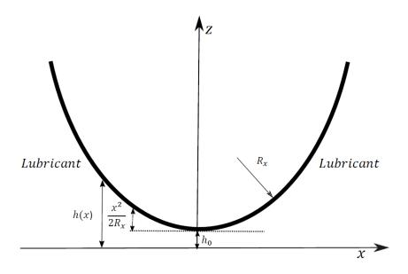
Figure 2.6: Fully flooded lubrication regime
