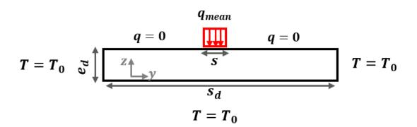
Figure 2.10: 2D liner thermal model
