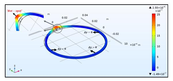
**Figure B.2:** Ring surface deformation as a result to the temperature variation (see figure B.1) (3D model analysis)
