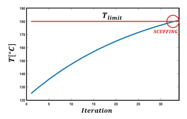
Figure 4.9: Temperature evolution over the thermo-mechanical loop
