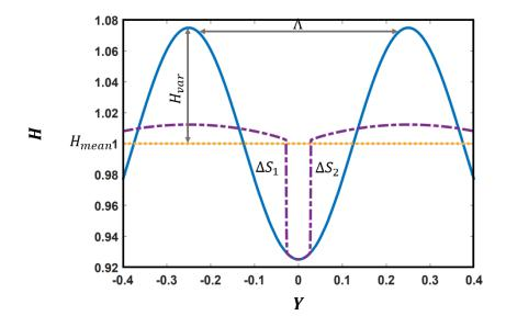
Figure 3.14: Lubricant distributions before and after the ring passage
