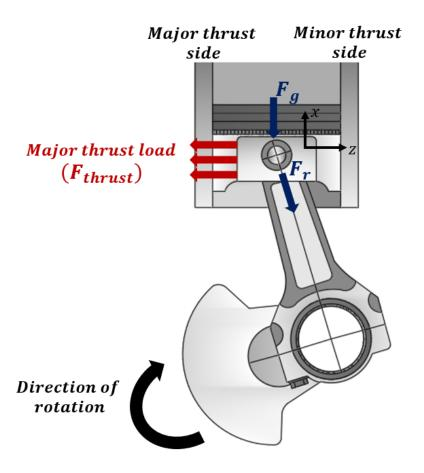
**Figure 3.3:** Power stroke phase of the engine
