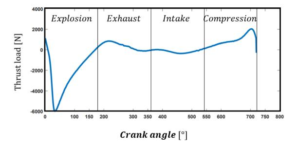
Figure 3.20: Thrust load distribution for an engine cycle
