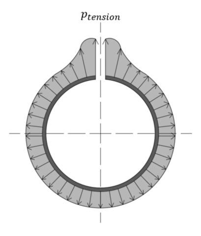
Figure 3.2: Radial pressure pattern of a piston ring
