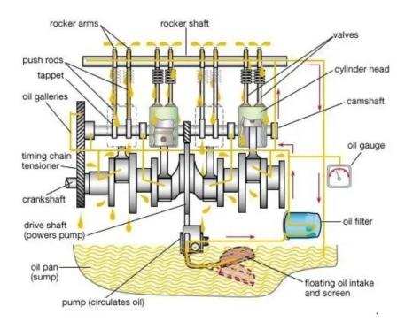
Figure 1.1: Lubrication circuit of an ICE [3]
