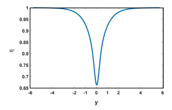
Figure 3.7: Dimensionless lubricant viscosity distribution
