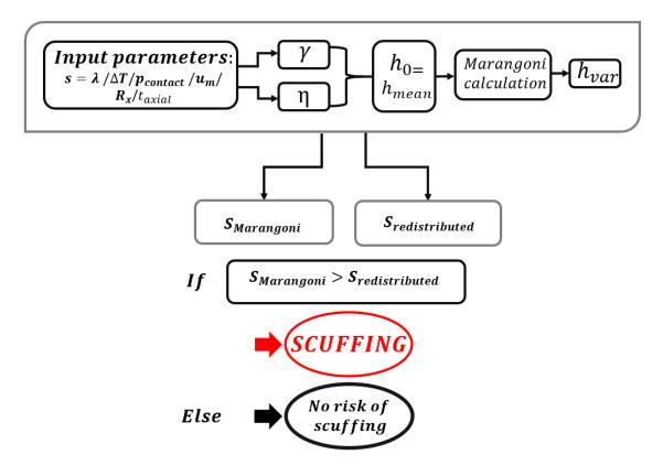
Figure 3.1: Lubricant distribution model
