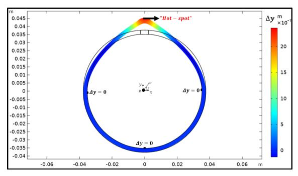
**Figure B.5:** Ring surface deformation as a result of the temperature variation (see figure B.4) (2D model analysis)
