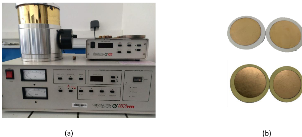
Figure 2.3. (a) Sputter coater for gold electrode coating; and (b) samples with circular gold electrode of 20 mm diameter.
