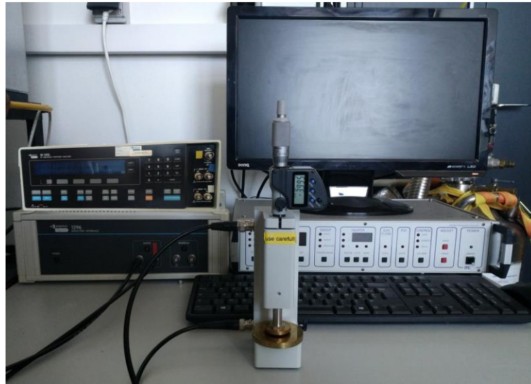
Figure 2.14. Experimental setup for dielectric characterization
