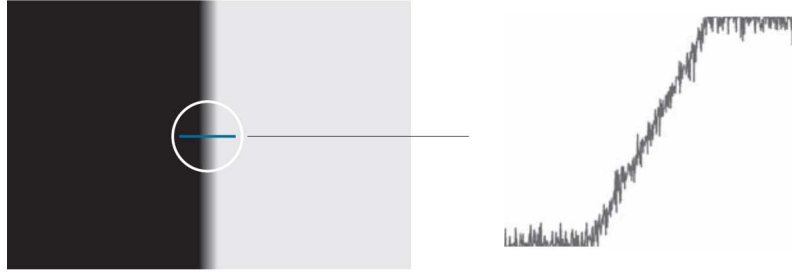
Figure II.6: Two regions separated by a blurred edge in a digital image. Source: [76]
