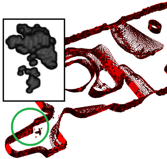
Figure II.3: Shrinkage cavities inside a CT volume after applying a segmentation algorithm that separates discontinuities from the background.
