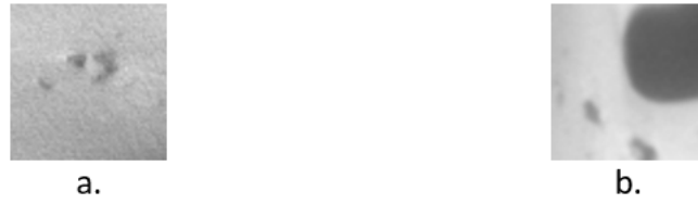
Figure IV.4: Two types of defective images in the dataset: (a) defect surrounded by a uniform background, (b) defect surrounded by a uniform background and a dark zone outside the casting body.
