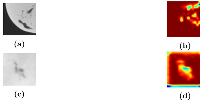
**Figure IV.9:** Grad-cam output of the final convolutional layer showing the class trigger: (a-c)  $64 \times 64$  zones with shrinkage cavities; (b-d) Grad-CAM by CT-Casting-Net.
