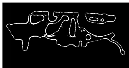
Figure II.11: The same fudge factor does not give good results for all slices of the same volume. As the thickness changes along the volume, the X-ray absorption changes and so does the contrast of the images. Therefore, the fudge factor must be adjusted independently for each slice.
