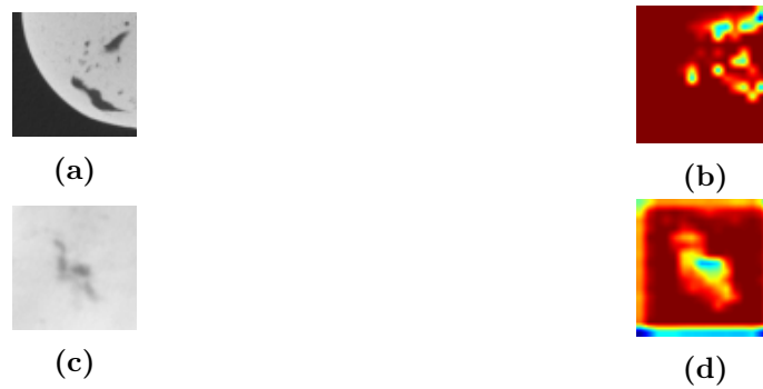
Figure IV.9: Grad-cam output of the final convolutional layer showing the class trigger: (a-c) 64 \times 64 zones with shrinkage cavities; (b-d) Grad-CAM by CT-Casting-Net.
