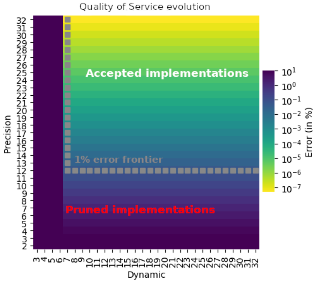
Figure 6.7: Quick pruning strategy for Quality of Service based exploration on the dot product meta design †† (considering vectors of 8 elements)
