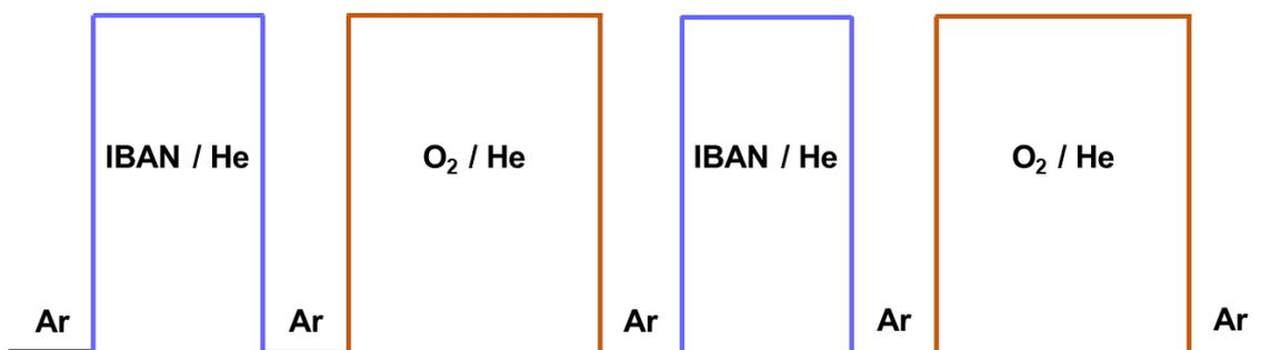
**Figure 2.7** Schematic diagram of alternating flow of reactant and oxidant in a periodic system.
