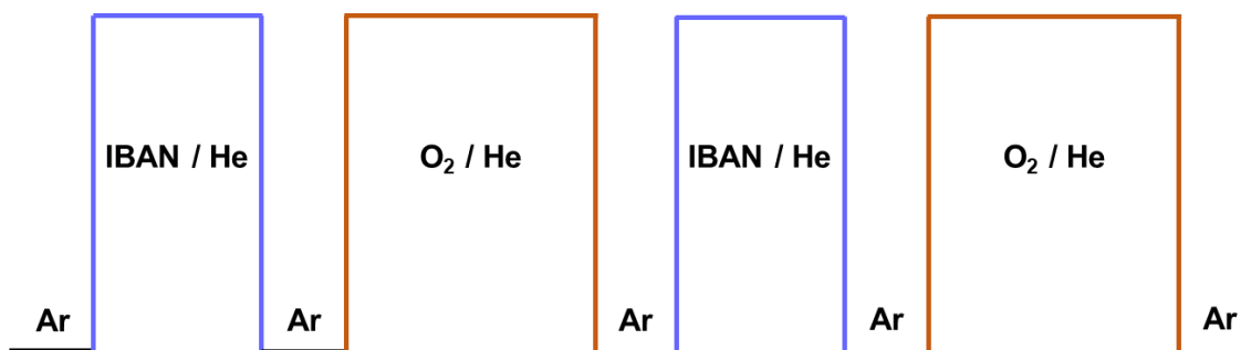
Figure 2.7 Schematic diagram of alternating flow of reactant and oxidant in a periodic system.
