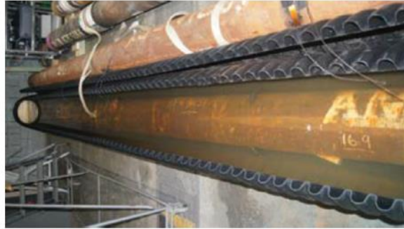
Fig. 4. Experimental setup for analyzing the response of a cylindrical pipe immersed in water.
