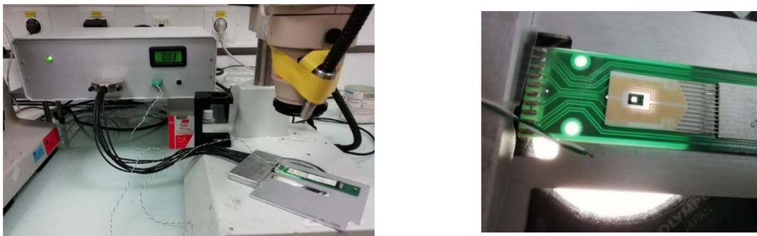
Figure 4.18 Process of sample preparation. Left - Nanocalorimetry chip with a chip holder is placed under the microscope and connected to the Nanocalorimeter in order to perform sample preparation, right – close view of the nanocalorimetry chip under the microscope.
