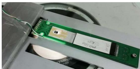
**d.** Chip holder with a nanocalorimetry chip for sample manipulation under microscope
