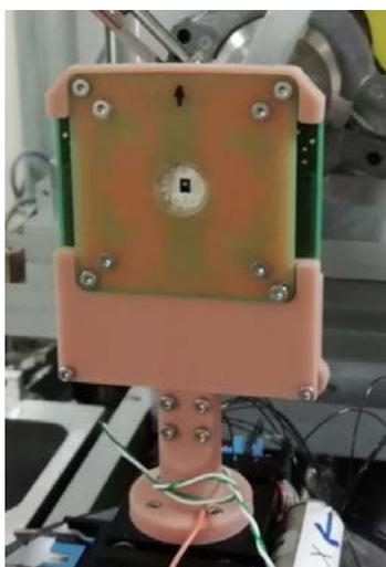
**c.** Chip holder with a nanocalorimetry chip with ceramic housing for measurements in-situ with X-ray micro-diffraction
