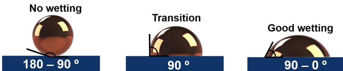
**Figure 2.4-3** Illustration of the different wetting behaviors.
