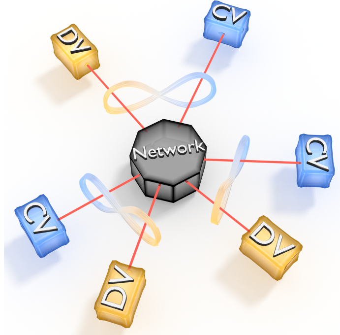
Figure 3.11: A heterogeneous quantum network. The connection of DV (yellow) and CV (blue) quantum nodes is made possible by optical hybrid entanglement.
