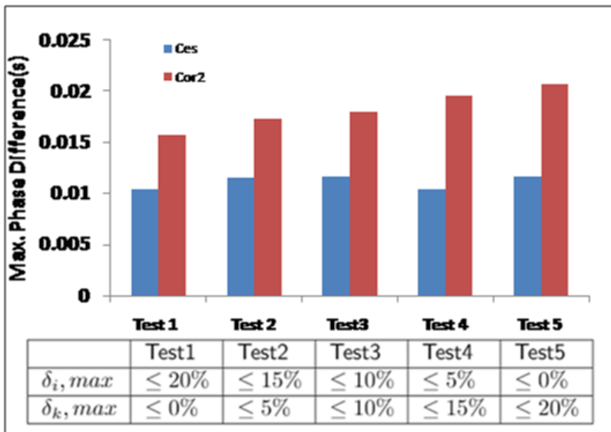
Figure 11.5: The figure shows the average phase difference under different values of \delta_i and \delta_k . The error of Corr^2 increases with the increase in \delta_k unlike C_{es}
