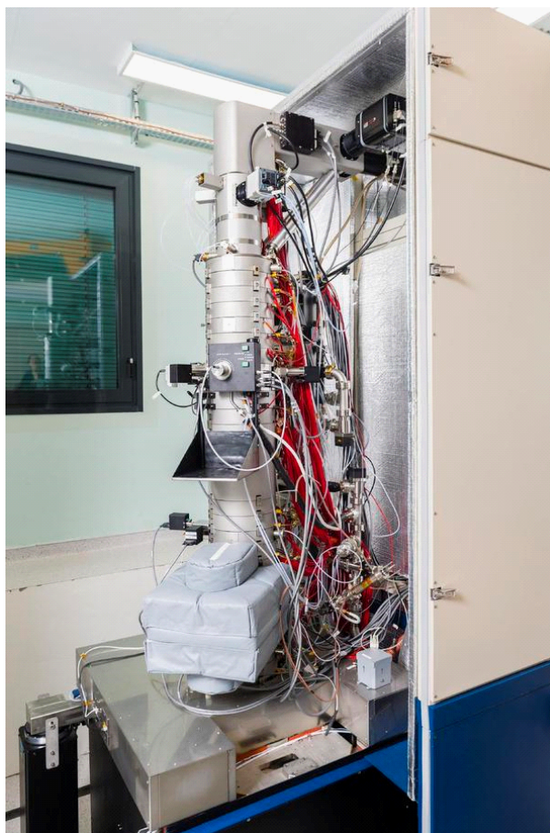
Figure 2.19: ChromaTEM: picture of the ChromaTEM, the monochromator is inside the grey fabric box.
