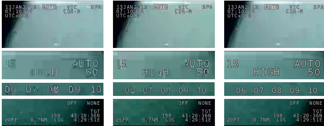
Figure 3.7: Reconstruction artifacts for the class-A color decoded video at QP=50. Left: HEVC; Center: SCC; Right: our proposed scheme.
