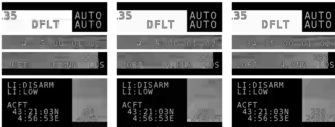
Figure 3.8: Reconstruction artifacts for the class-A grayscale-0 decoded video at QP=50. Left: HEVC; Center: SCC; Right: our proposed scheme.
