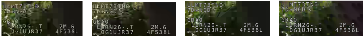
Figure 5.11: Reconstruction artefacts at QP=50 for Prop-Inter. From left to right: HEVC-SCC (PSNR 25.86 dB), VVC (PSNR 26.45), Prop-HEVC (PSNR 27.07 dB) and Prop-AVC (PSNR 26.1 dB).
