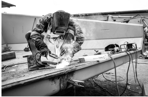
FIGURE 1.1 – Soudage SAEE - Document W. Roche.
