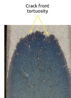
Figure 3.21: Details of the crack front tortuosity on the spec. S4-F4 at 700°C.
