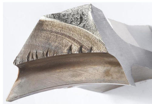
(a) Schematic view of the fatigue cracking process. (b) Example of a gas turbine blade failed under fatigue.
