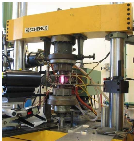
(a) Overall view of the 63 kN Schenck testing machine (from [Kaminski, 2007]).
