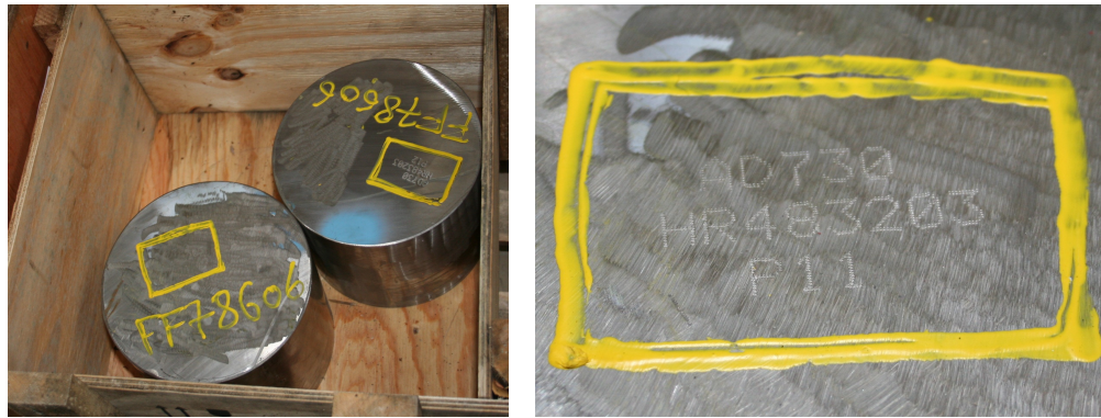
(a) As-received raw material of AD730™ in the form of two Ø 204 mm cylinders.
