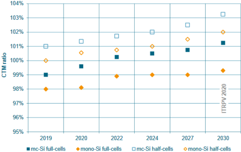
Figure 14: Trend of cell-to-module (CTM) power ratio for the next ten years as forecasted by the ITRPV 2020.
