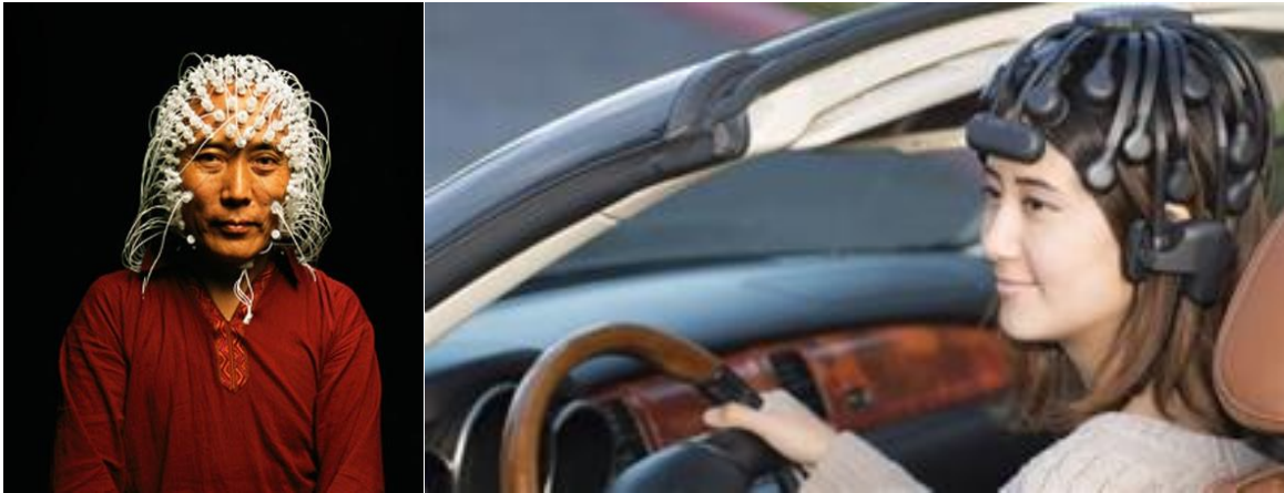
Figure 10. Illustration of the technological innovations in EEG technology. Left: High-density, research-grade, stationary 128-channel EEG system. Source: National Geographic (2009). Right: Wearable, wireless, 32-channel EEG system Source: Cognionics (2021).
