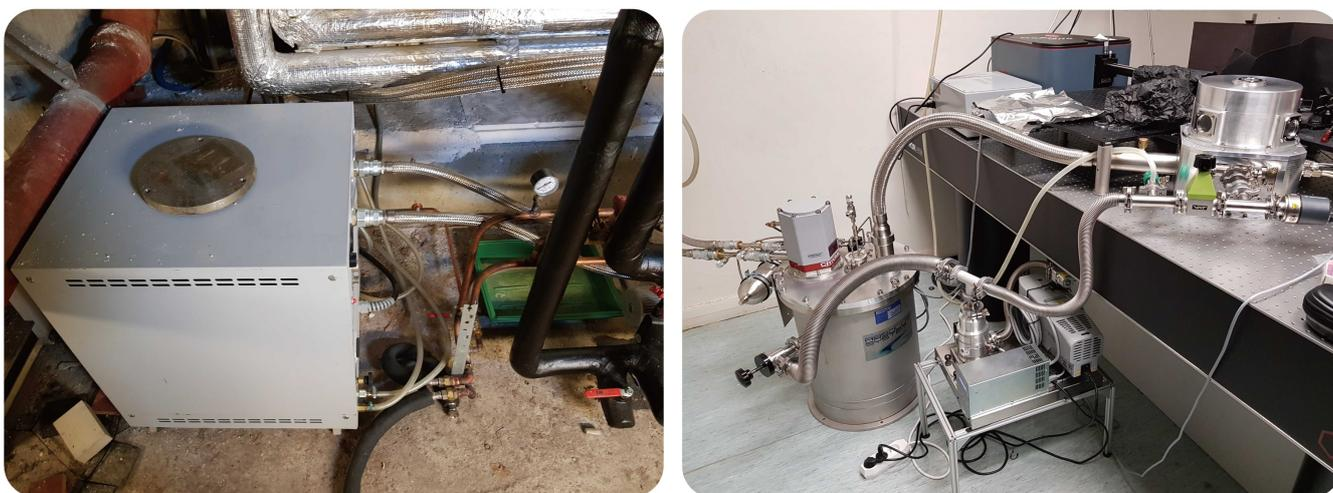
Figure 2.19: Optical images of (left) the helium compressor and (right) the cryostat.
