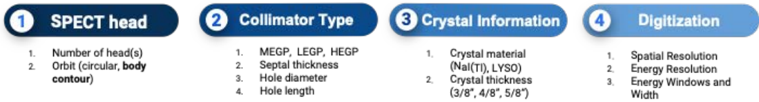
Figure 5.3: Schematic of modelling the gamma camera components and its response
