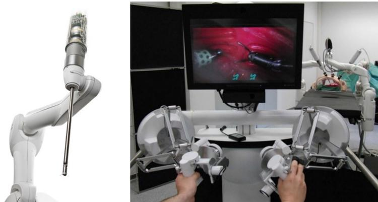
FIGURE 2.3: 7 DOF MiroSurge robot and its 6 DOF joystick [Tobergte et al., 2011].
