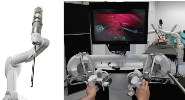
FIGURE 2.3: 7 DOF MiroSurge robot and its 6 DOF joystick [Tobergte et al., 2011].
