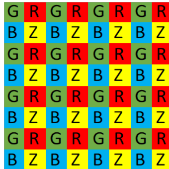
Figure 4.11: Representation of the Mask1: RGB-Z matrix based on the Bayer pattern built using the 1x1-Z-pixel.
