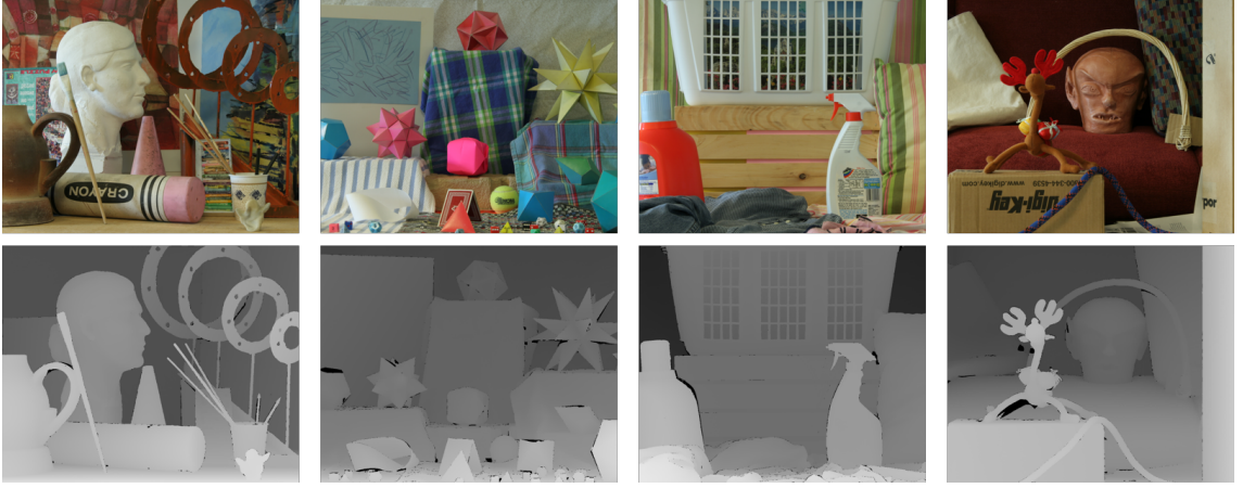
Figure 4.9: Four examples of color images and their associated disparity map from Middlebury database [23][24].
