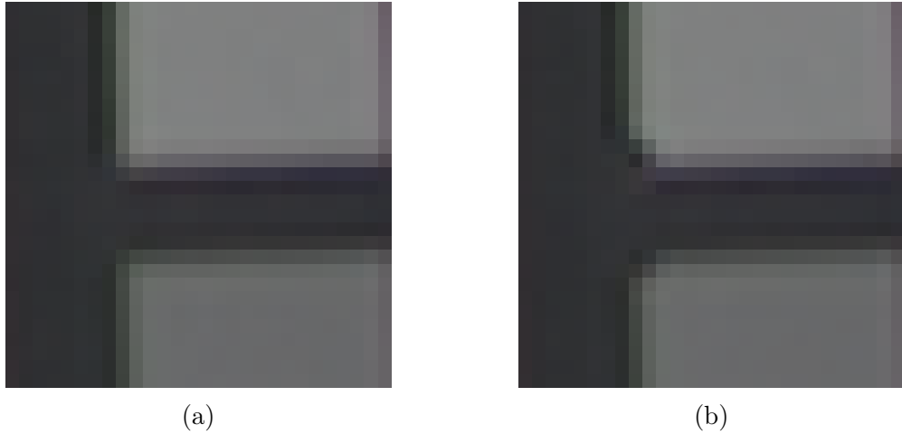
Figure 4.20: Example of reconstruction errors of a corner for Mask2 architecture. (a) Reference image. (b) Reconstructed image using semi-gradient method. The image is a crop from the CAVE database [27].
