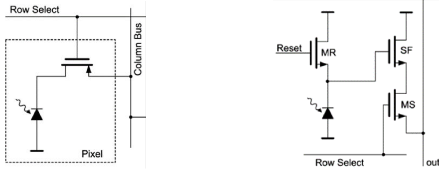
Figure 1.2: Schematic of two types of CMOS pixel [1]. (a) PPS. (b) 3T-APS.
