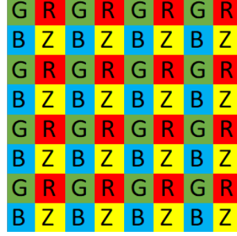
Figure 3.3: Representation of the Mask1: RGB-Z matrix based on the Bayer pattern built using the 1x1-Z-pixel.
