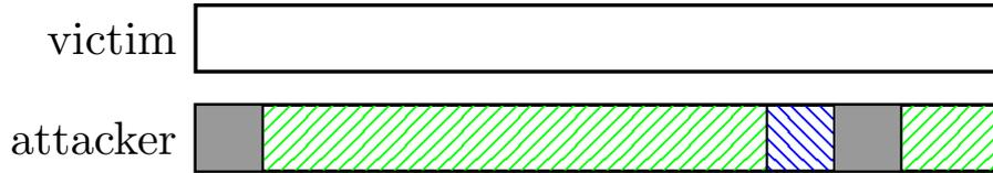
(b) The attacker fills the cache with her addresses, evicting the monitored address. The victim does not access the monitored address. The attacker's addresses are still in the cache. The attacker accesses her addresses again, and the access time is reduced.
