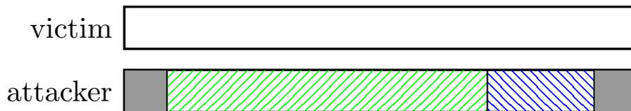
(b) The attacker flushes the probed address from the cache. The victim does not access the address. The attacker accesses the address, and the access time is high.
