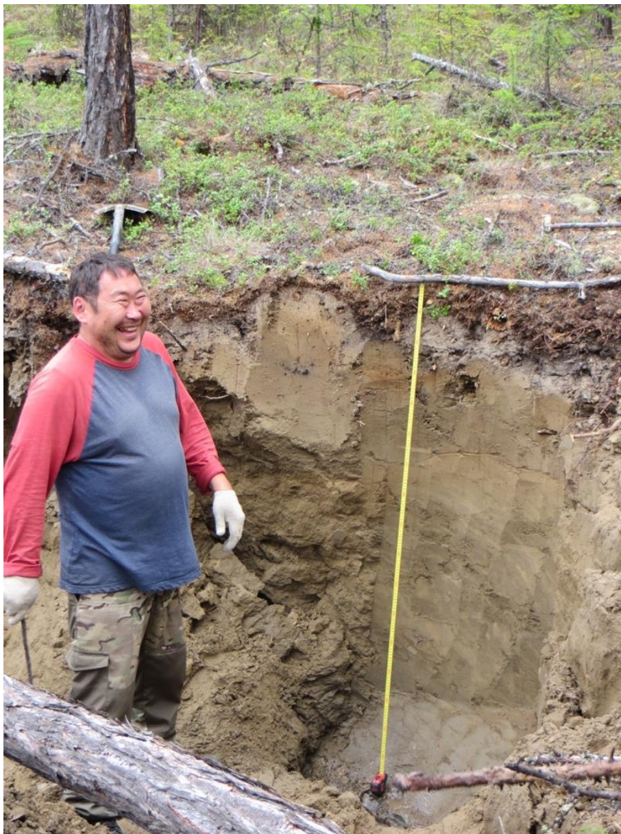
Figure 3. Active layer in a forested area near Syrdakh village (Sakha Republic). Frozen ground is visible below the tape measure.
