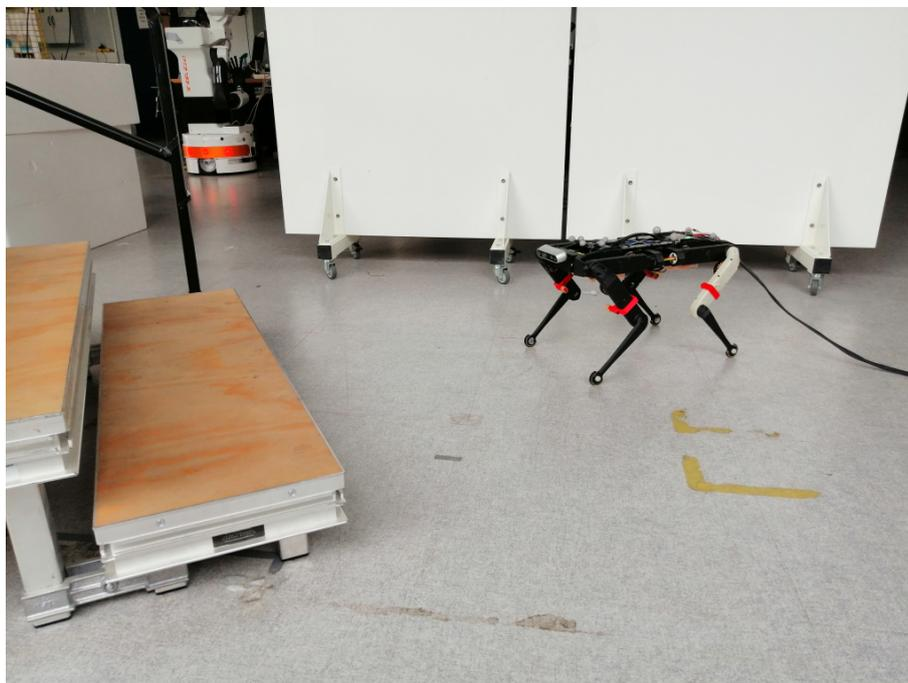
Figure 10.1: Experimental setup: a RealSense D435i is mounted on the Solo robot that localizes itself with respect to stairs. A motion capture system provides ground truth of the robot pose.
