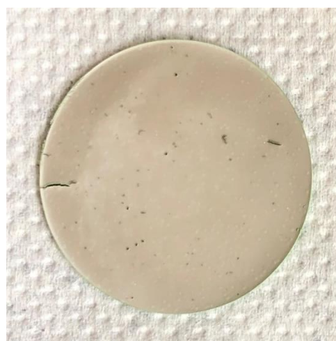
Figure E.1: Pictures of half-cell after co-sintering, the electrolyte layer is on the top side
