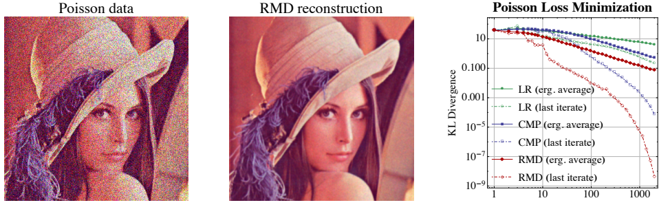
Figure 5.1: Reconstruction of the Lena test image from a sample contaminated with Poisson noise. Left to right: (a) the contaminated sample; (b) RMD reconstruction; and (c) Poisson likelihood loss at each iteration. The RMD process provides a sharper definition of image features relative to the CMP algorithm (which is the second-best).
