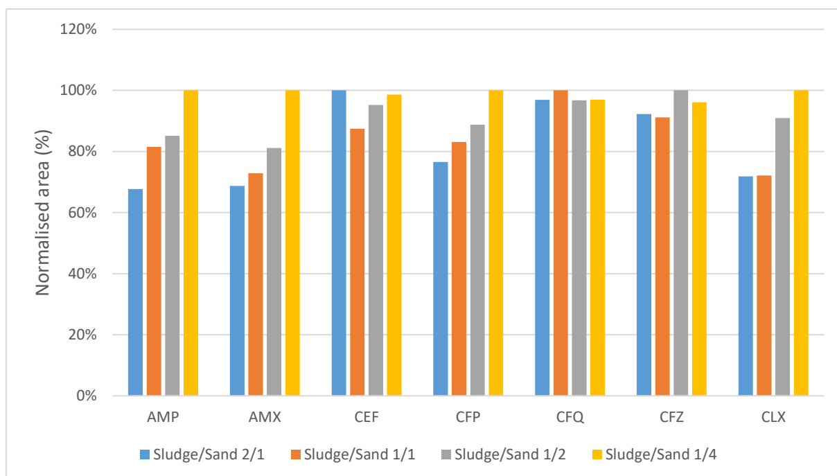
Figure 3 : Normalized area obtained for the extraction of the analytes with various sludge/sand ratio (500 mg sludge; extraction solvent: 5 mL H 2 O and 10 mL ACN).
