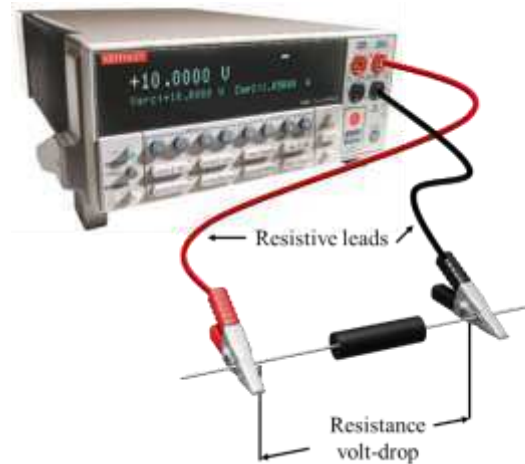
Figure 2.13 Two-wire measurement usually plugin lead resistance affecting measurement accuracy.
