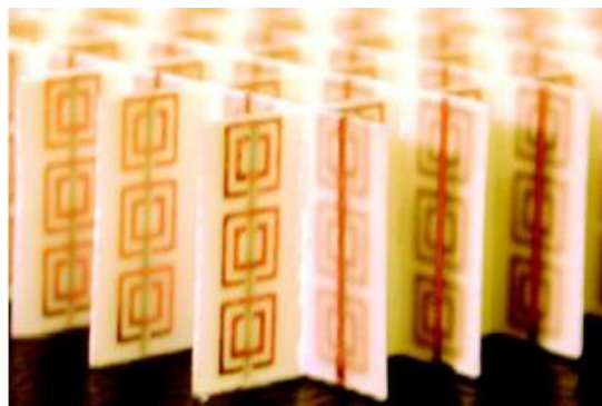
Figure 1.2 Photograph of the left-handed metamaterial (LHM) sample [4] .
