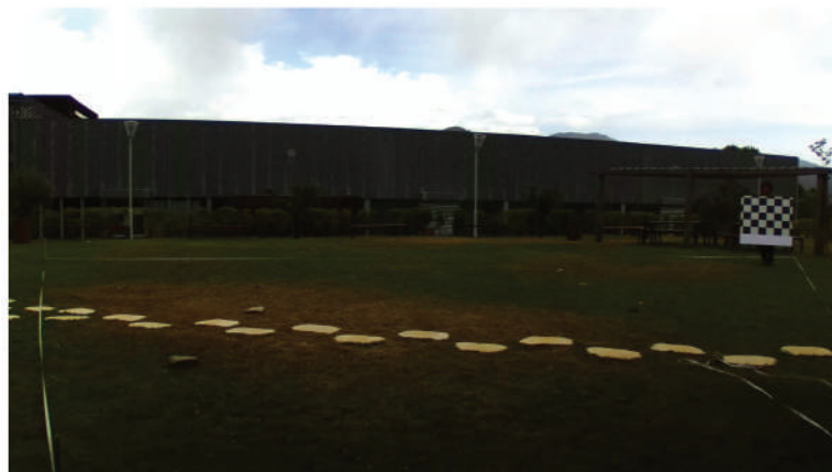
Figure 4.3: Image of the checkerboard with a distance camera-target equal to 12 m.
