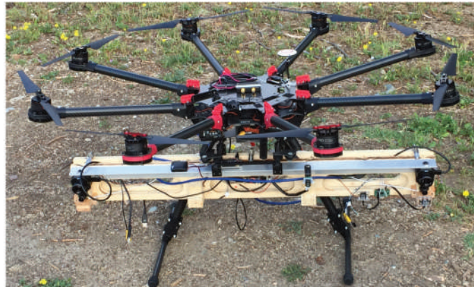
Figure 2.12: Visible and infrared stereovision systems mounted on the drone DJI S1000.
