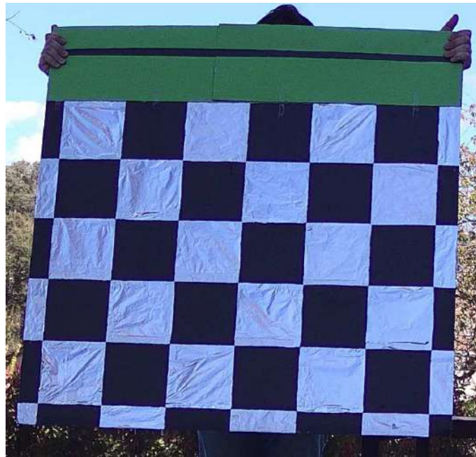
Figure 4.7: Image of the checkboard modified to be visible by the LWIR cameras.
