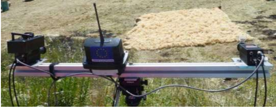
Figure 1.19: System developed by Toulouse et al. : two cameras that work in multimodal bands (near infrared and visible), on the left there are the IMU sensors, and in the middle there is the receiver to start the cameras [54].
