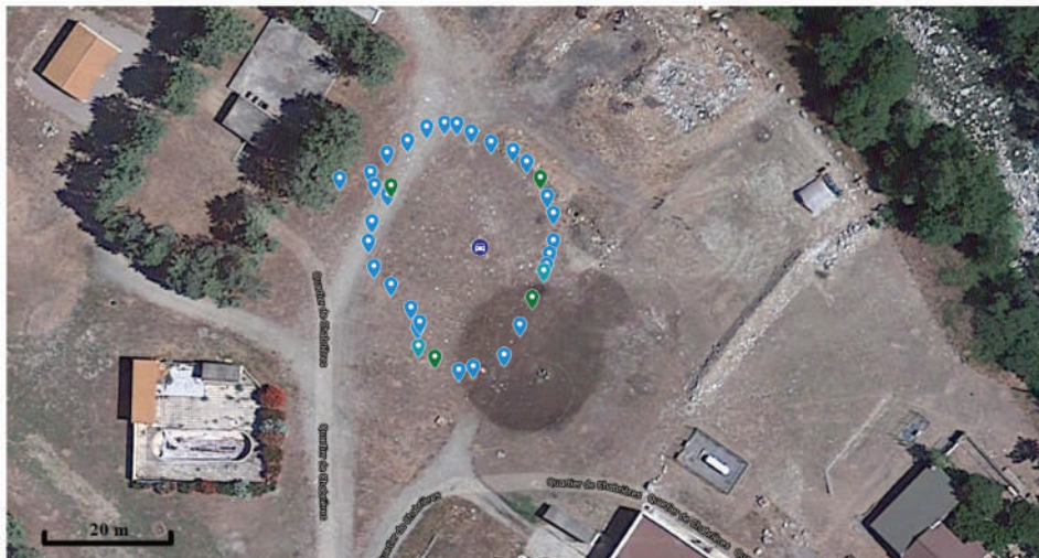
Figure 5.2: Drone and car positions registered by GPS sensors. The light blue icons represent the positions of the drone during the test, the green icons represent the positions of the drone when the picture is captured. The dark blue icon represents the position of the car.
