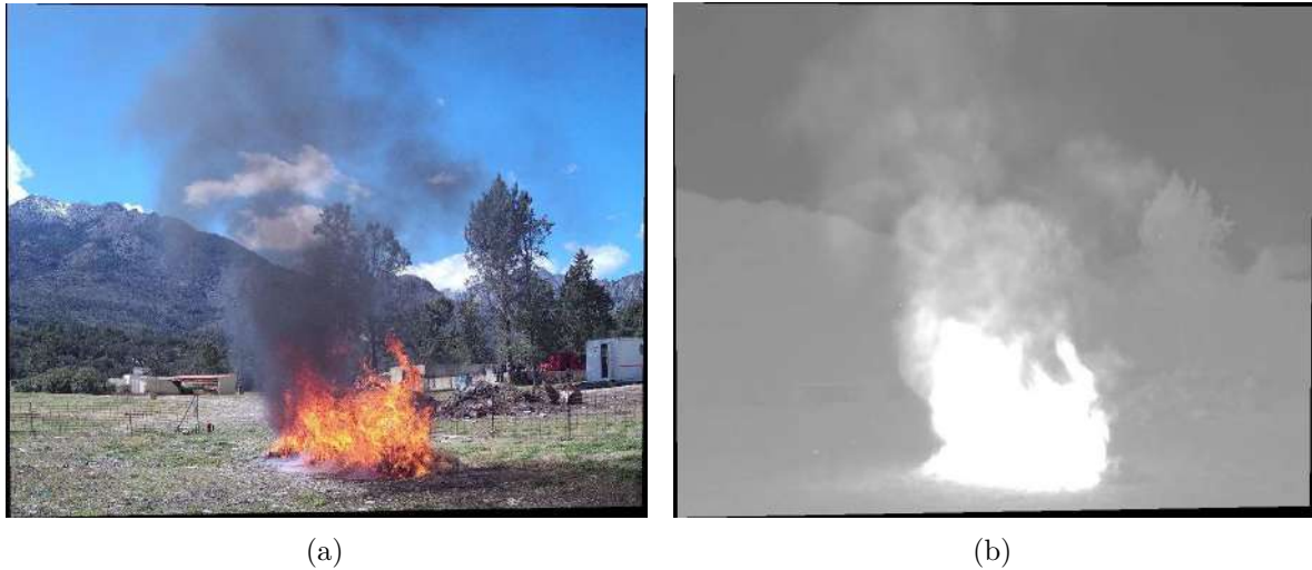
Figure 2.6: Fire images obtained simultaneously in the visible and LWIR spectra. (a) visible image. (b) LWIR image.
