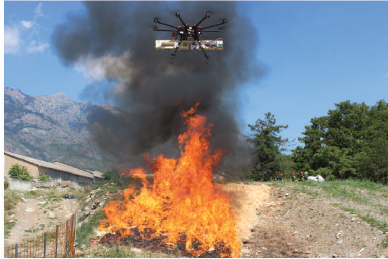
Figure 2.9: Vision system carried by the DJI S1000 UAV located at the rear of a fire approximately 12 m away.
