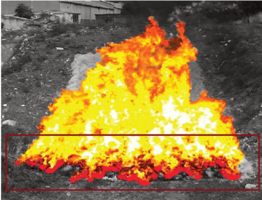
Figure 4.34: Example of ground fire pixels selected by the proposed method (red crosses).
