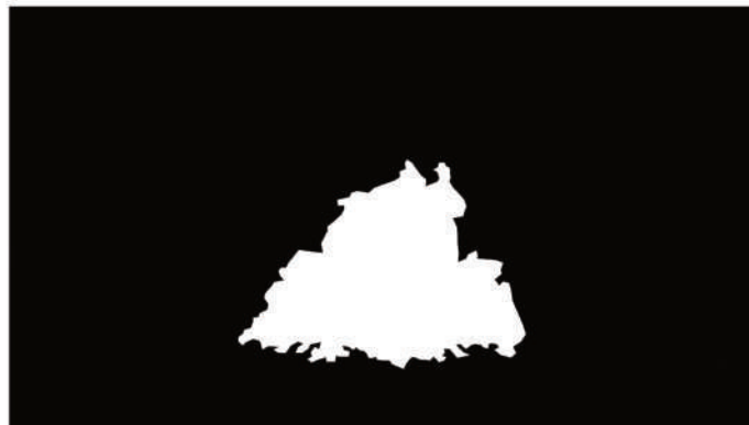
Figure 4.15: Example of the binary mask of the fire image (in white are the pixels of the fire zone, in black are the pixels of the background).
