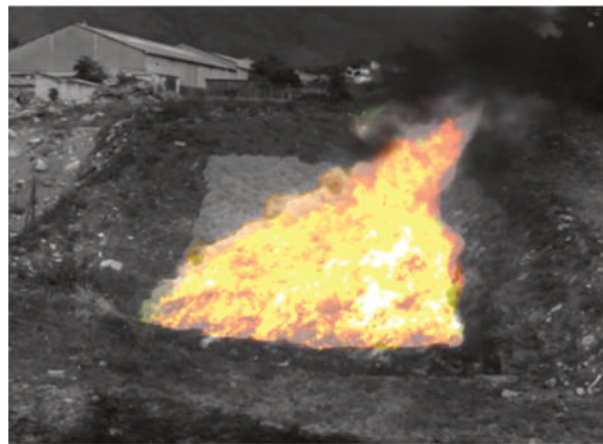
Figure 4.11: Fire zone detected in the LWIR image used as a pre-selected area in the visible image.
