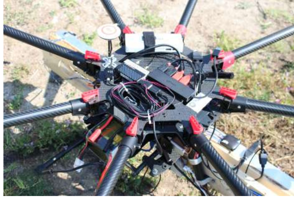
Figure 2.21: Drone mounting the material for power and for video transmission to the ground.
