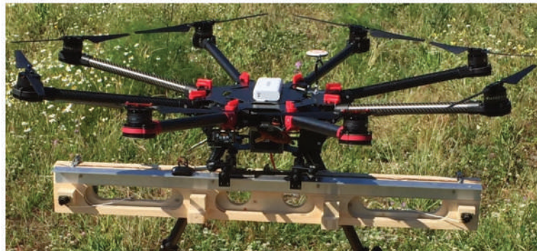
Figure 2.8: Visible stereovision system mounted on the drone DJI S1000.
