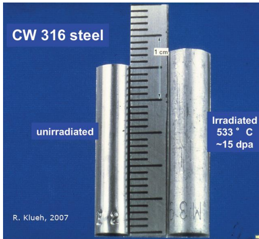
Figure 39 – Swelling (effect of vacancy clustering) of CW 316 steel (Klueh, 2008).
