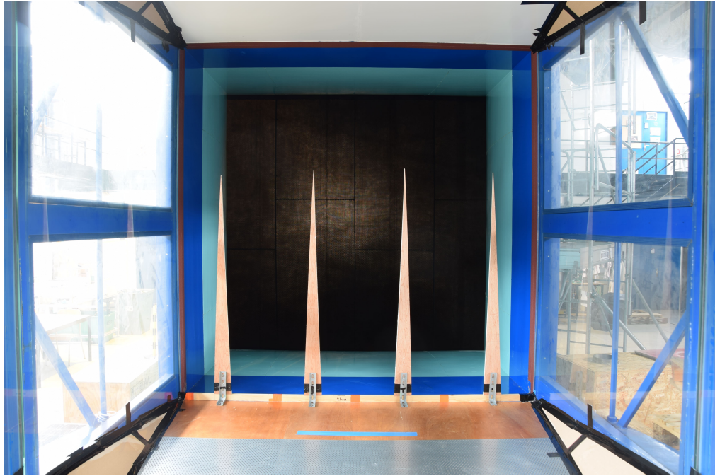
Figure 3.13 – Turbulence generation at the LHEEA atmospheric wind tunnel facility. A trip and spires placed at the end of the wind tunnel’s convergent are used. Perforated metal plates are placed on the ground to enhance small scale turbulence development. The beginning of the corner fillets are also visible in the corners of the wind tunnel.
