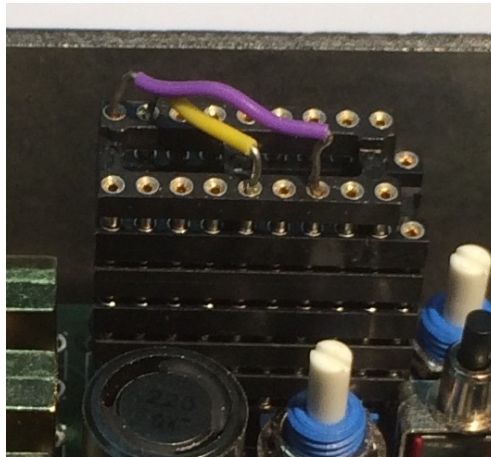
FIGURE D.2 – Câblage du Coala
