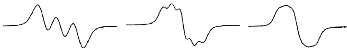
Figure SIII.44 EPR signals measured by Lancaster et al. for triarylamine-based radical cations 51 . (left) Three-line pattern, corresponding to unpaired electrons localized on one triarylamine; (center) five-line pattern, ascribing to unpaired electrons partially delocalized between two triarylamines; (right) one-line pattern, attributing to unpaired radicals fully delocalized without energetic barrier to the charge transfer.
