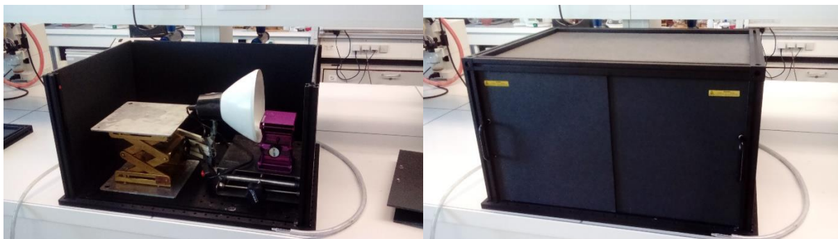
Figure SIII.42 Photographs of the (H) 23-W Philips halogen classic warm white 204 lumen lamp, placed in an opaque box to block the surrounding light during irradiations.
