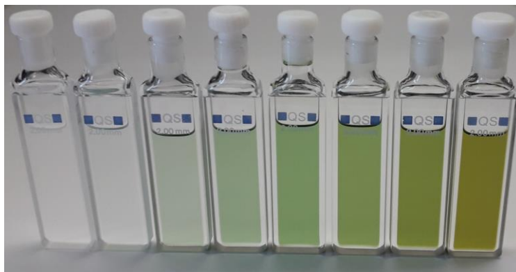
Figure III.20 Picture showing solutions of TATA-C12 at 2.3 mM in \text{CHCl}_3 after dissolution then after 10s, 45s, 90s, 180s, 360s, 720s and 1440s of light irradiation (from left to right). The solution was irradiated in a 2 mm rectangular quartz cuvette by the setup A, with a surface optical power of 7.9 \text{ mW/cm}^2 .
