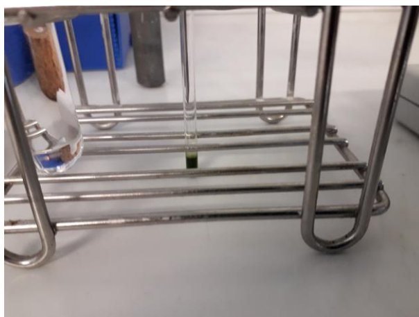
Figure SIII.53 EPR tube containing the thin film of a light irradiated TATA-C12 solution at 2.3 mM in chloroform. The film formation was carried out upon nitrogen flushing. The solution was irradiated in a 2 mm rectangular quartz cuvette by the setup A, with a surface optical power of 7.9 \text{ mW/cm}^2 .
