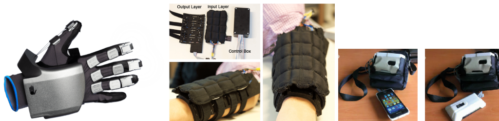
Figure 2.2 – The SenseGlove Nova, a vibrotactile sleeve (TaSST, by Huisman et al.) and the Dialtact system (Lenay et al.)
