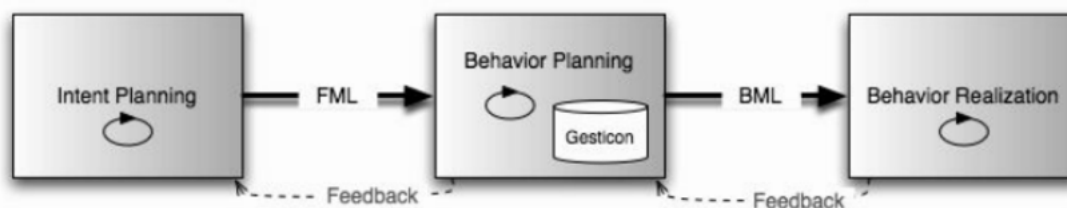
Figure 6.1 – The SAIBA model of behaviour animation planning and realization
