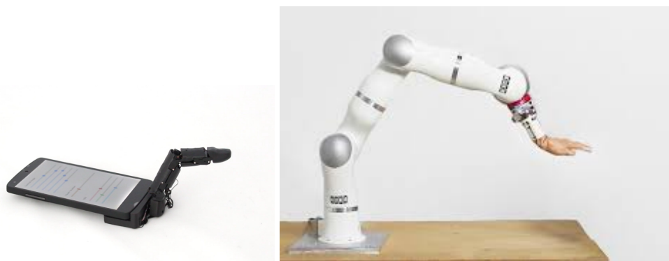
Figure 2.1 – Examples of tangible haptic devices (Mobilimb on the left, and a robotic arm on the right, both by Teyssier et al.)
