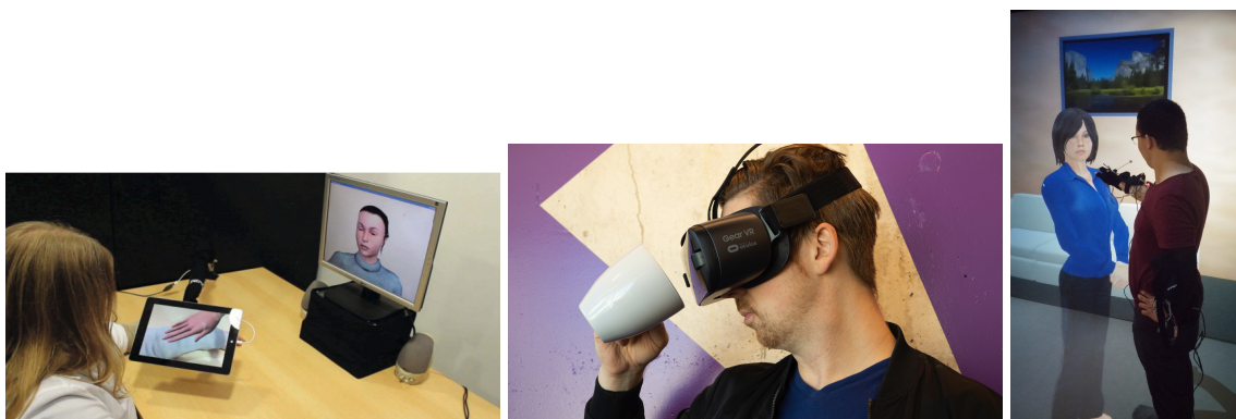
Figure 3.2 – Augmented reality (left), virtual reality (middle) and immersive room (right) setups
