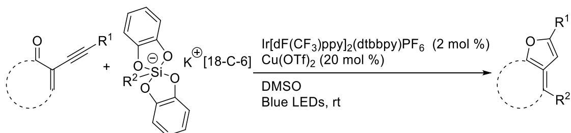
Scheme 65. Cu/photoredox catalyzed cycloisomerization of 2-alkynyl-cyclohexenones
