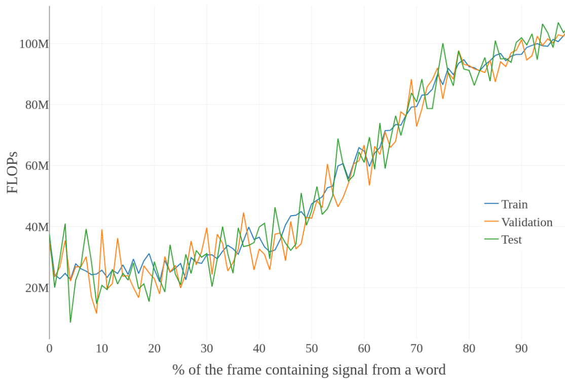
Figure 4.11. – Average number of FLOPs required to evaluate the sampled models in function of the signal contained in the corresponding frame. We observe that model is able to effectively adapt its size, sampling simple models when the frame contains only background noise and leveraging more computation power when the frame contains an actual word.
