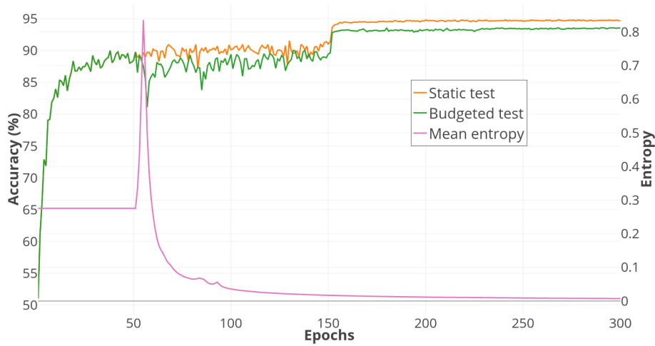
Figure 3.13. – Evolution of the loss function and the entropy of \Gamma during training. The period between epoch 0 and 50 is the burn-in phase. The learning rate is divided by 10 after epoch 150 to increase the convergence speed.
