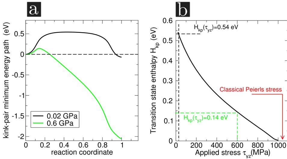
Figure 3.3: **Kink pair nucleation enthalpy.** (a) Minimum enthalpy path associated with the nucleation of a kink-pair, at two different levels of stress. (b) kink pair nucleation enthalpy as a function of the applied stress. All curves were obtained with Provile potential. Reproduced from Provile et al. (2012) (Supp. Materials).
