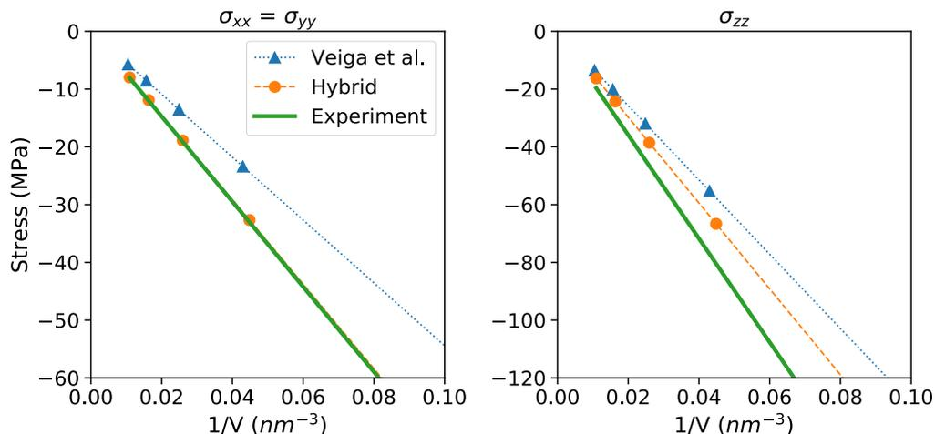
Figure 2.12: **Stress induced by the insertion of a carbon atom in an octahedral site as a function of the inverse volume of the simulation cell.** Experimental data are from (Schultz, 1968). Symbols correspond to our MD simulations. Dashed lines are linear regressions.
