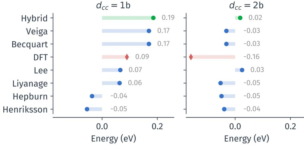
Figure 2.11: **Carbon-carbon binding energy in bulk iron as a function of carbon spacing  $d_{cc}$  in the [111] direction.** Values obtained with different interatomic potentials are compared to *ab initio* data (Becquart et al., 2007).
