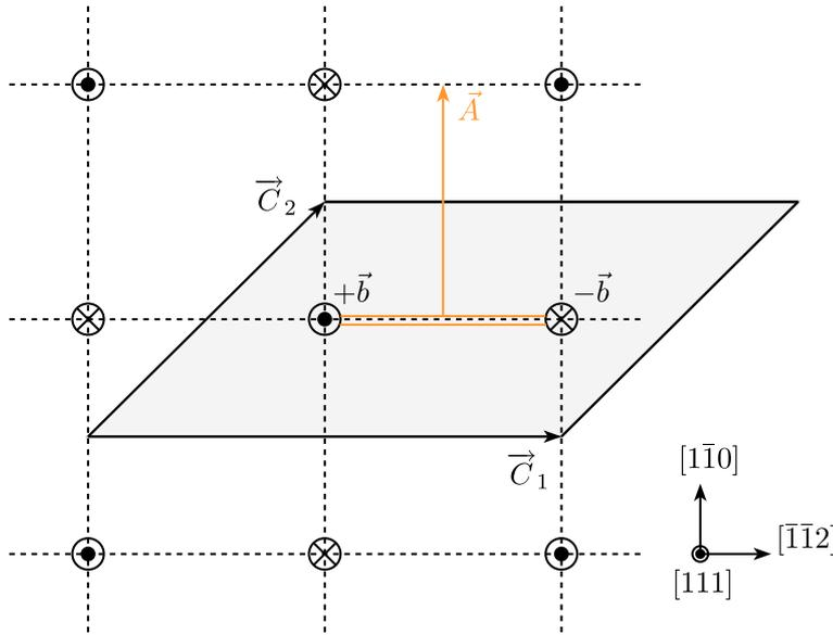
Figure 1.1: **Quadrupolar arrangement of dislocations typically used in DFT simulations.** The simulation cell (grey shape) contains two dislocations of burgers  $+\vec{b}$  and  $-\vec{b}$ . Figure extracted from (Ventelon, 2008).
