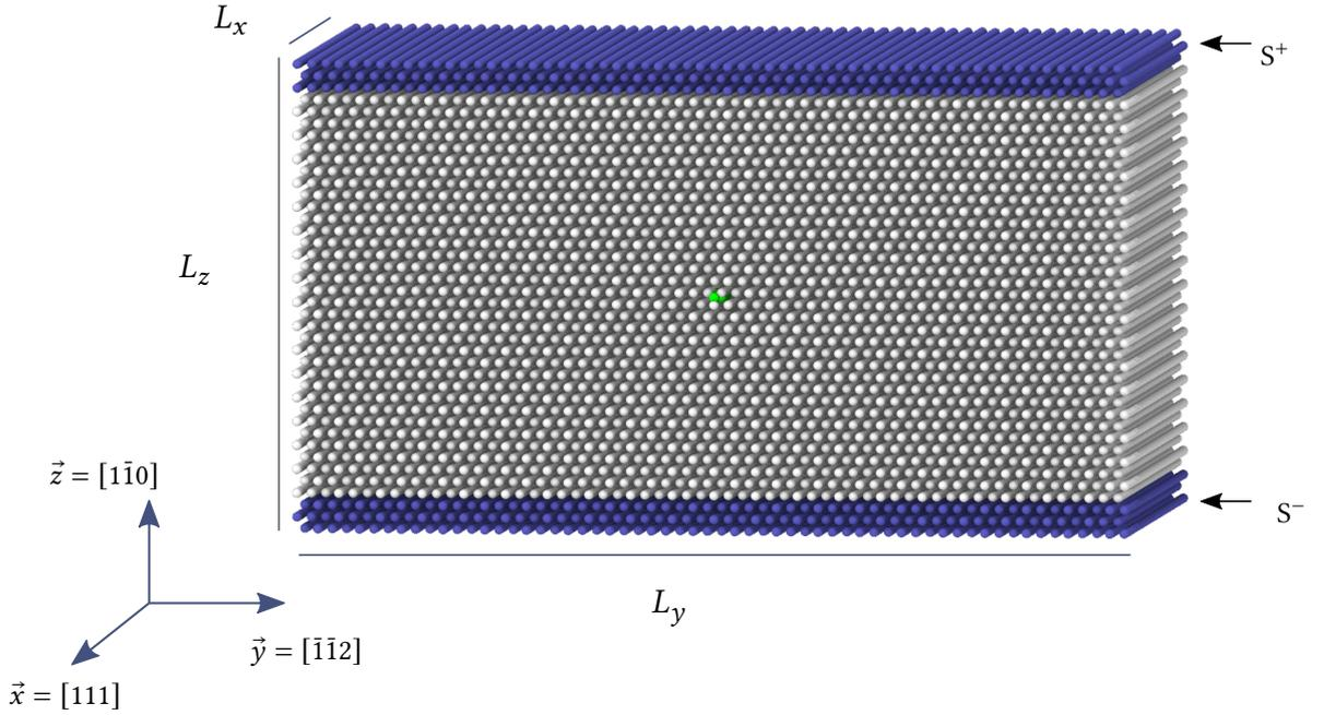
Figure 1.2: **Simulation cell used for dynamical simulations.** A screw dislocation (indicated by a green line) is inserted along the  $[111]$  direction in the middle of a crystal of bcc iron. Two regions denoted  $S^\pm$  are used to shear the crystal (in blue). Atoms visualization was obtained with Ovito.
