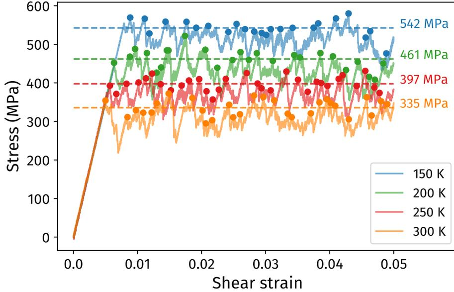
Figure 3.5: **Typical stress-strain curves from MD simulations, at different temperatures.** Simulations conducted with Provile potential with an imposed shear rate  $\dot{\gamma} = 1 \times 10^7 \text{ s}^{-1}$ . Stress peaks are represented by circles. A dashed line represents the average of the peaks for each temperature (*i.e.* the computed flow stress).
