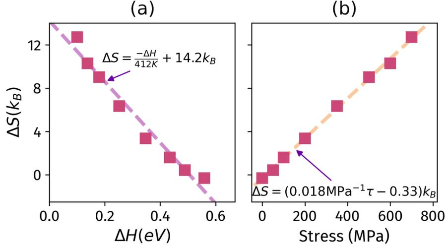
Figure 3.13: **Effective activation entropy  $\Delta S$  as a function of (a) the activation enthalpy  $\Delta H_{kp}$  and (b) the shear stress  $\tau$ .** The slopes of linear regressions of Fig. 3.12 are plotted as a function of the activation enthalpy in (a) and stress in (b) (square symbols), and fitted to: (a) an inverse Meyer-Neldel entropy-enthalpy relation (Eq. 3.18), (b) a linear stress-activation entropy relation.
