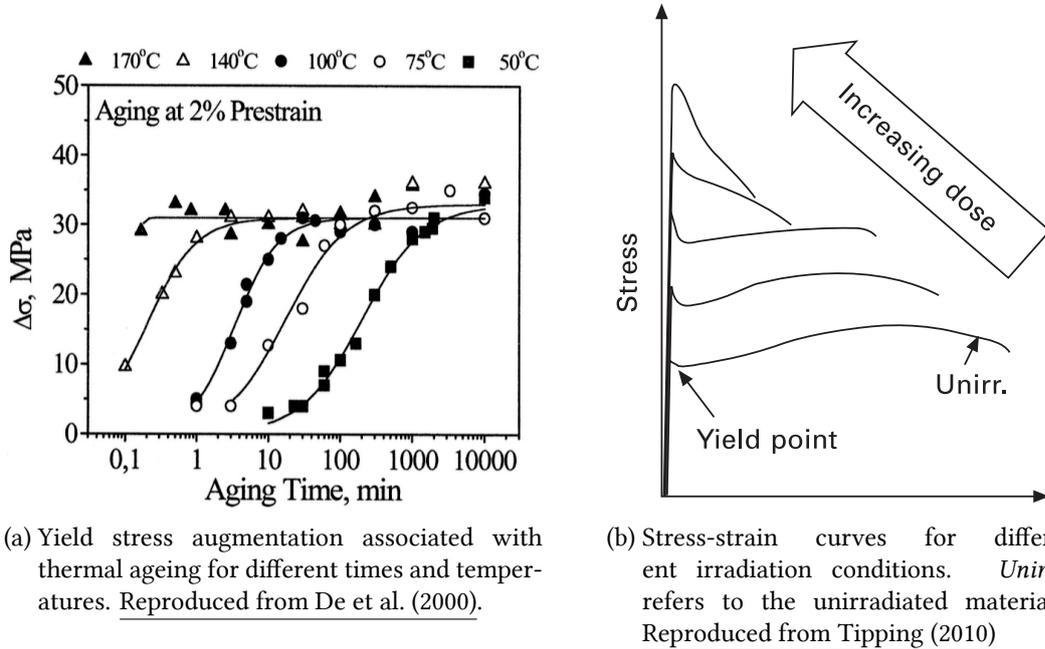
Figure 0.2: **Effect of thermal ageing and irradiation on ferritic steels.**
