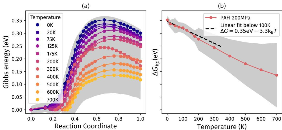
Figure 3.11: **Minimum Gibbs free energy paths associated with the nucleation of a kink pair under 200 MPa in Fe, at different temperatures.** (a) MGEP profiles: PAFI free energy data (symbols) and corresponding splines (lines). (b) Temperature evolution of the Gibbs energy of activation. A linear regression in the domain below 100 K is shown as a dashed line. Both plots share the same y-axis.
