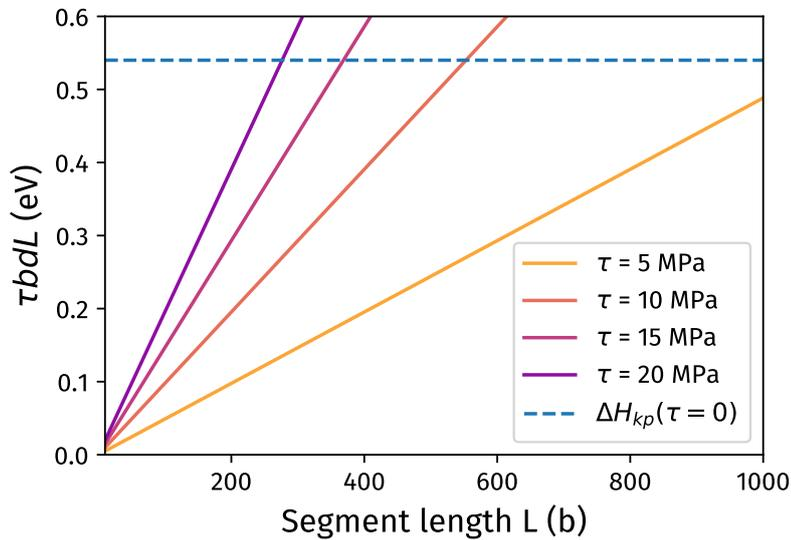
Figure 3.6: **Evolution of the plastic work  $\tau b d L$  as a function of  $L$ , for different values of  $\tau$ .** For comparison, a dashed line represents the upper bound for  $\Delta G_{kp}$  i.e. the zero-stress enthalpy  $\Delta H_{kp}(\tau = 0)$  (see Fig. 3.3).
