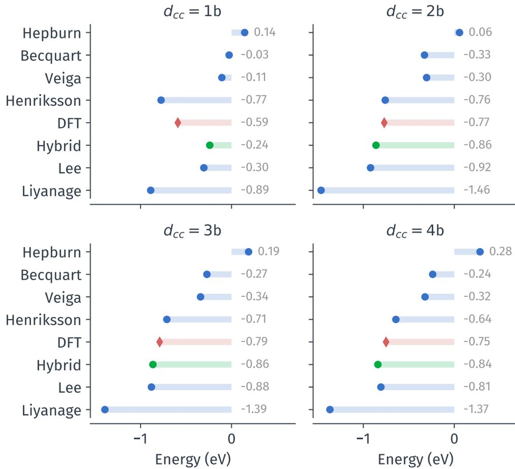
Figure 2.10: **Carbon-dislocation binding energy, as a function of carbon spacing  $d_{cc}$  along the dislocation line.** Values obtained with different interatomic potentials are compared to *ab initio* data (Lüthi, 2017). Horizontal lines serve as guides for the eye.
