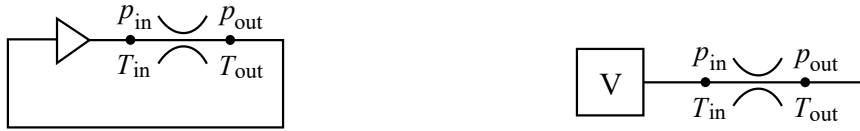
(a) Closed cycle with warm compressor (b) Open cycle with high-pressure storage
