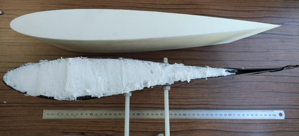
FIG. IV.10 Pattern of resin profile NACA0012 with a chord of 400 mm and the corresponding test sample.
