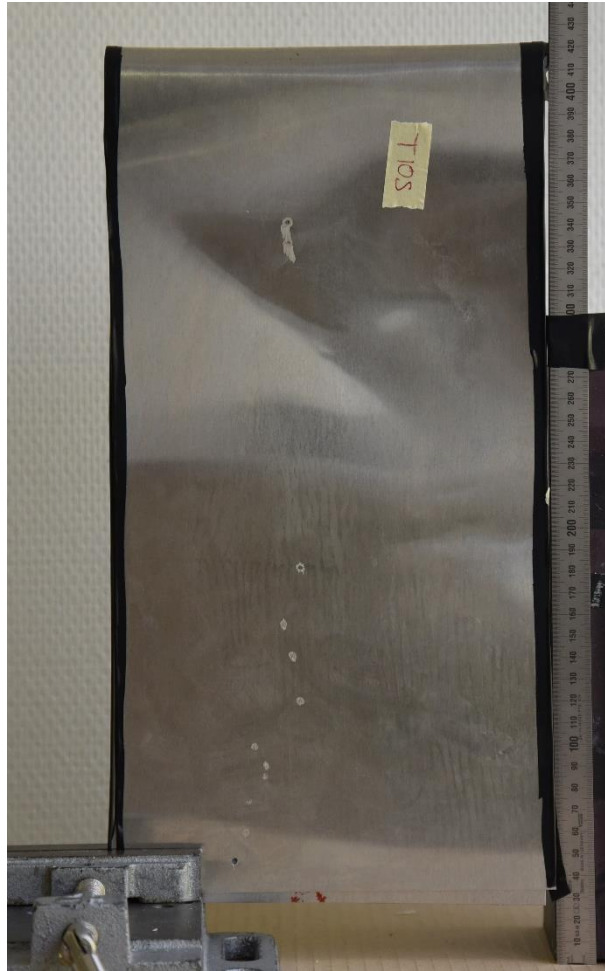
FIG. V.11 Presentation of different kinds of track left by cathodic arc root – normal end and discontinuous tracks (a) thinner end and continuous track (b) jumping tracks (c).
