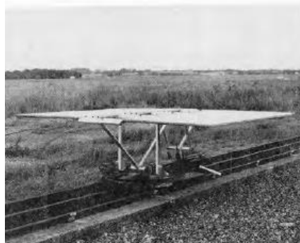
FIG. I.13 Different approaches to reproduce a swept-stroke with a moving electrode: the electrode is either propelled by a truck (a) (Plumer (2012)), a stretched elastic (b) (Plumer (2012)) or gas release (c) (Dobbing and Hanson (1978)).
