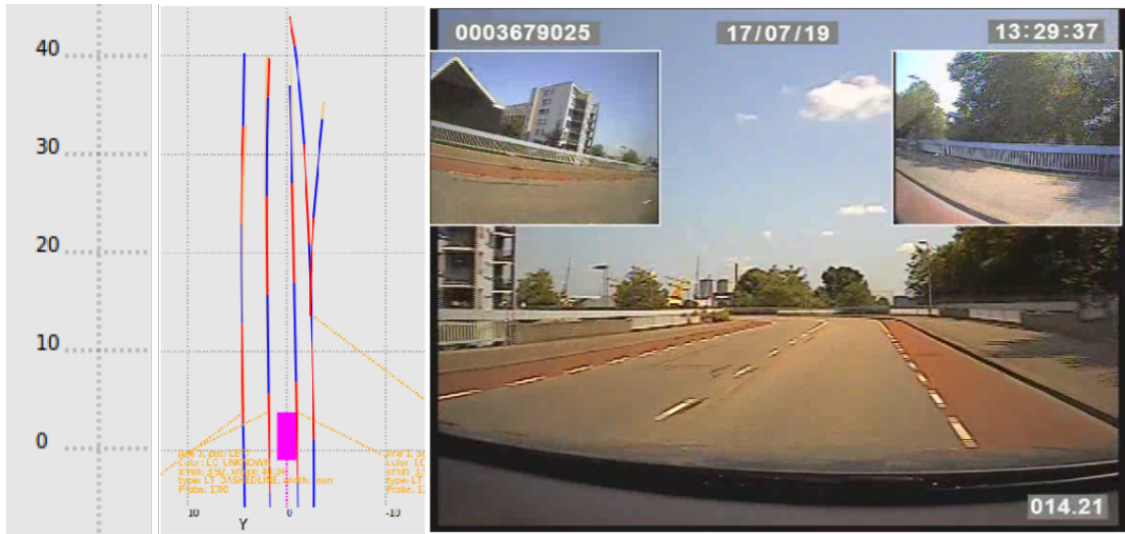
Figure 3.21: Left: tracking result (red and blue clothoid segments). Right: context camera. The fourth track from the left has been initialized from a FrontCam false detection. Noisy measurements are mistakenly accepted but correctly not associated to existing tracks.
