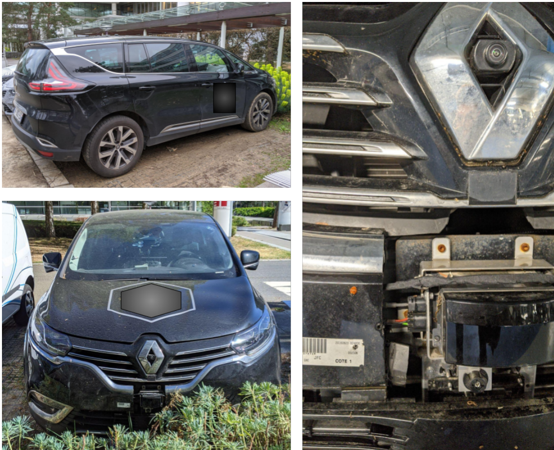
Figure 2.10: L3 prototype vehicle. On the left side of the illustration, the vehicle from two different viewpoints. On the right side, a detail of the front bumper featuring a front lidar and one of the sensors of the Smart AVM.
