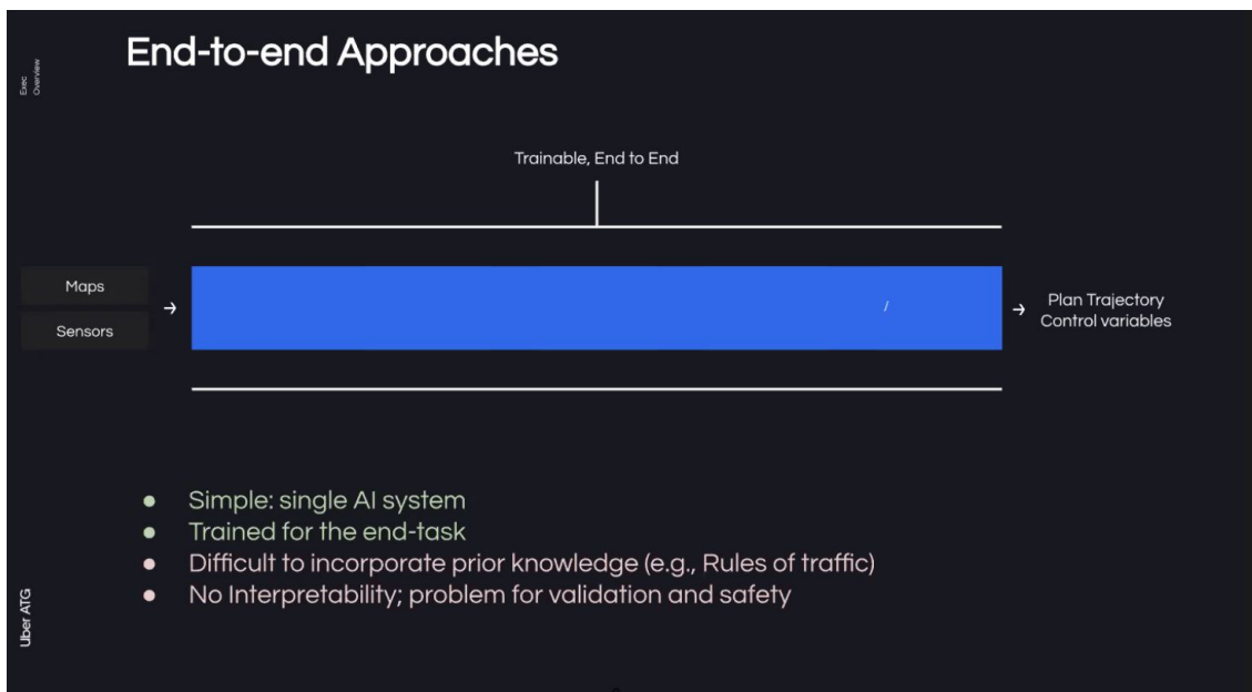
Figure 2.1: End-to-end [Urtasun, 2020] pipeline are completely learned architectures which are simple to be trained on the end task but hard to diagnose in case of (likely) issues in the general task.
